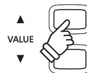
Alternatively, press the ▼ or ▲ VALUE buttons to cycle through all 9 different registration memories.
